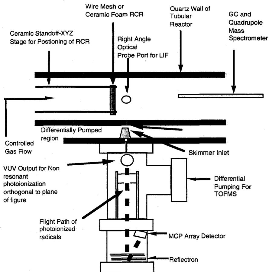
Figure 1 Schematic of experimental short contact reactor (Drawing not to scale).
