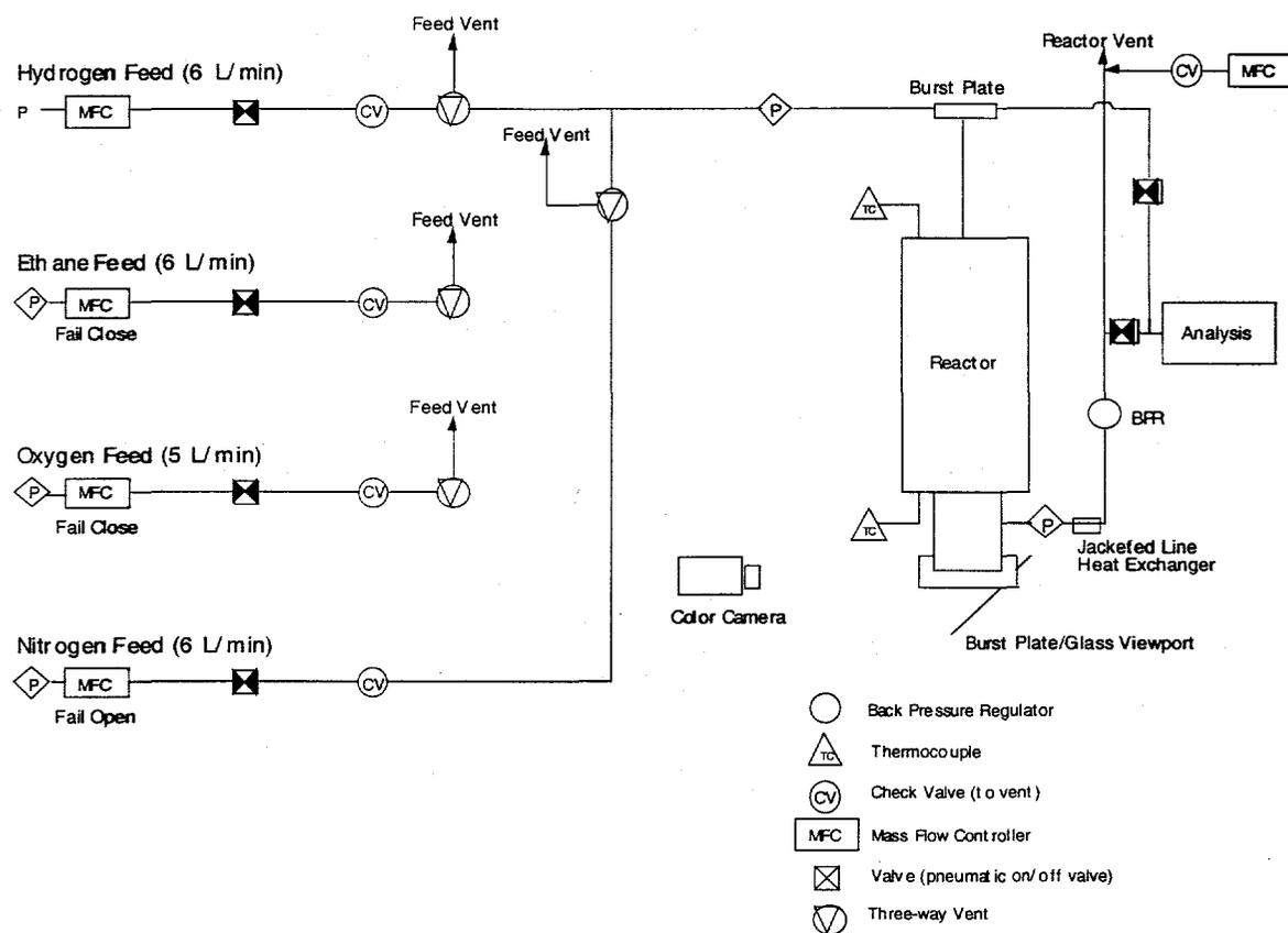
Figure 2 Schematic of overall experimental short contact reactor facility showing flow controls.
